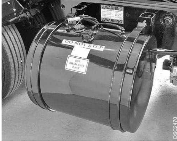
Fuel Tank and Fittings
